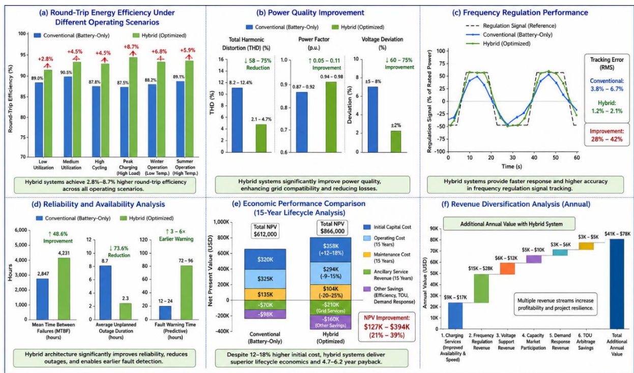
Figure 4. Comprehensive performance comparison between optimized hybrid battery-supercapacitor energy storage systems and conventional battery-only configurations.
