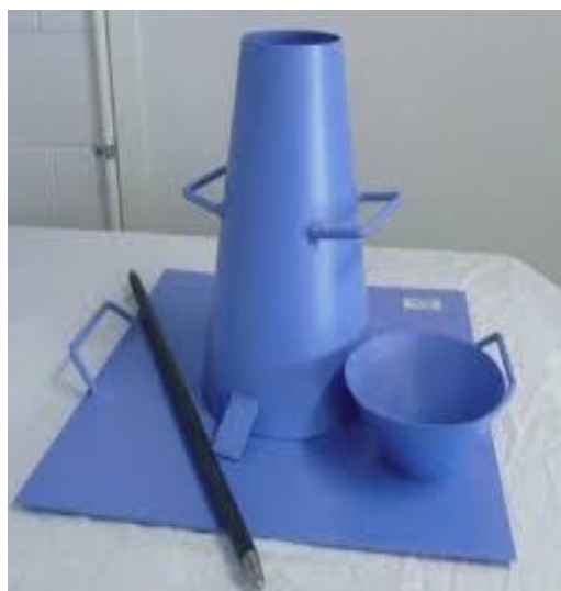
Fig 1: Slump cone test.
