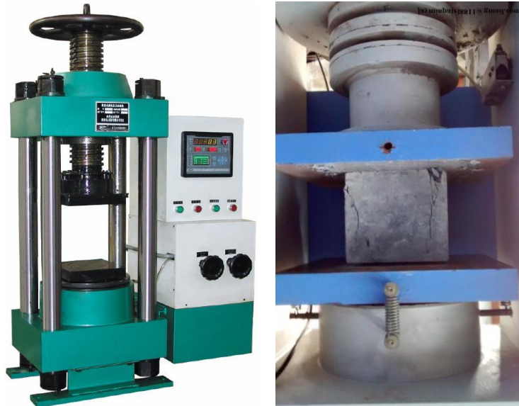
Fig 3: Compressive strength test.
