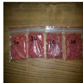
Fig 5: Samples of Step 3. (Boiling in Salt solution at 100°C for 30mins and 60mins)
