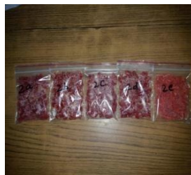
Fig 4: Samples of Step 2. (Boiling in Tamarind pulp and Water at 100°C for 60mins)
