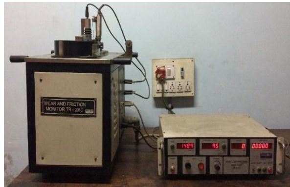
Figure 23: Pin on disc machine setup.
