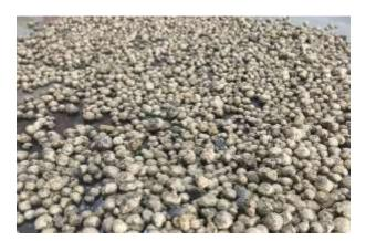
Fig 1: Fly ash aggregate.
