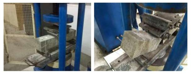
Fig 8: Flexural strengths on Beam.
