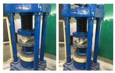
Fig 5: Split tensile strength on cylinder.
