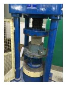
Fig 2: Compression strength on cube.
