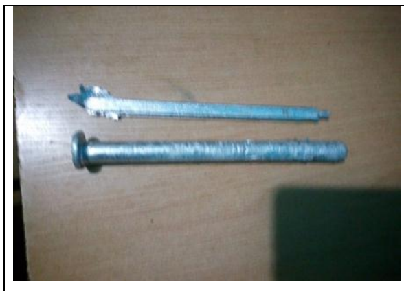
Figure 3: Sample of the Rectangular and Circular billet of the composite.
