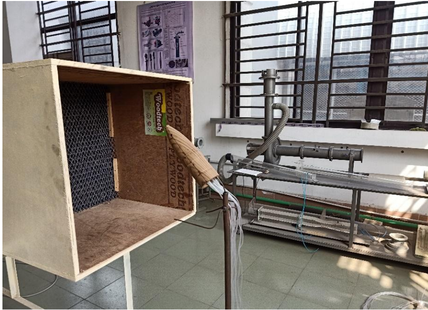
Figure 5: Experimental setup of 37 mm projectile for measuring static pressure.
