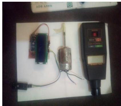
Fig. 5: The two tachometers with the 24VDC motor.
