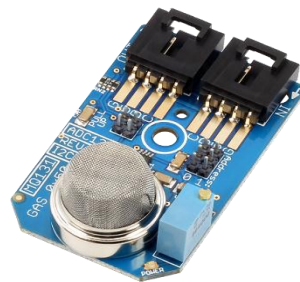
Figure 8: MQ131 Ozone gas sensor.
