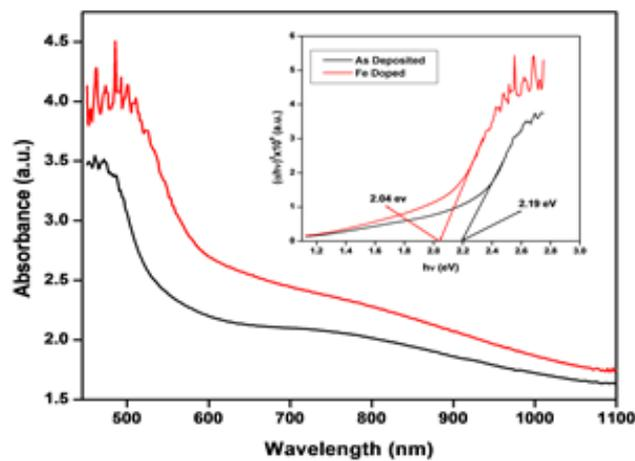
Figure 4: Shows the plot of wavelength against absorbance used for deriving the absorbance coefficient and inset figure represents the plot of energy against  $\alpha h\nu^2$  used for plotting the energy band gap of the materials.
