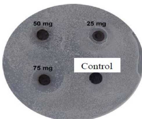
Figure 8: Determination of the antimicrobial effect of ZnFe_2O_4 -based nanomaterial on E.coli by diffusion susceptibility method (Experimental conditions: ^\circ T=25\text{ }^\circ\text{C} , Particle diameter=100 nm).
