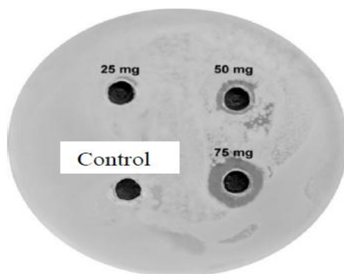
Figure 6. Determination of the antimicrobial effect of ZnFe_2O_4 -based nanomaterial on Bacillus subtilis by diffusion susceptibility method (Experimental conditions: T=25\text{ }^\circ\text{C} , Particle diameter=100 nm).
