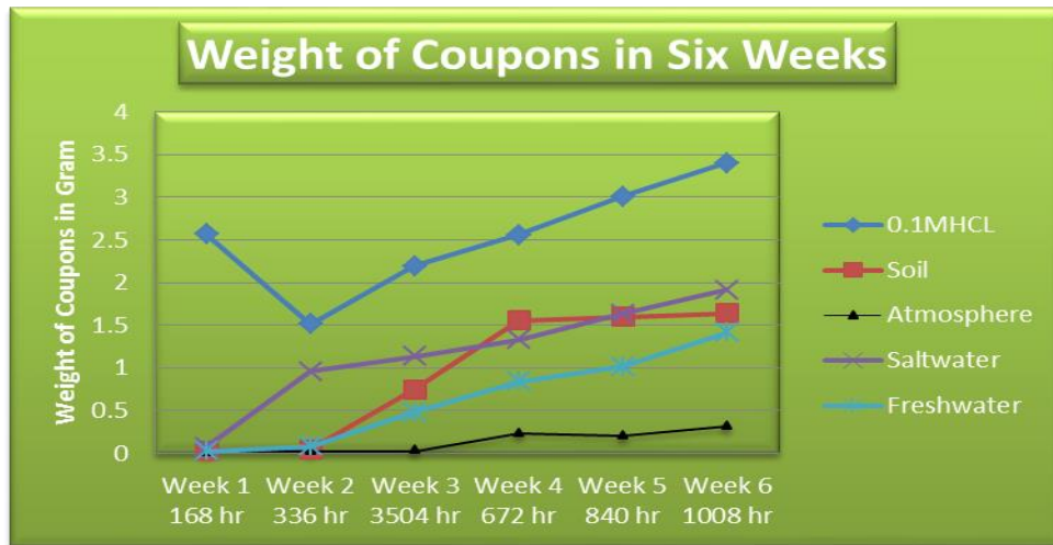
Figure 5: weight of coupons in six weeks.
