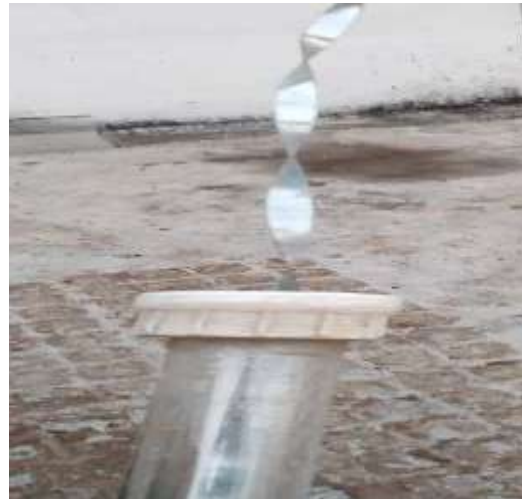
Figure 1: Full Length Evacuated Tube with Coupler. Figure 2: Twisted Tape Insertions in Evacuated Tube.
