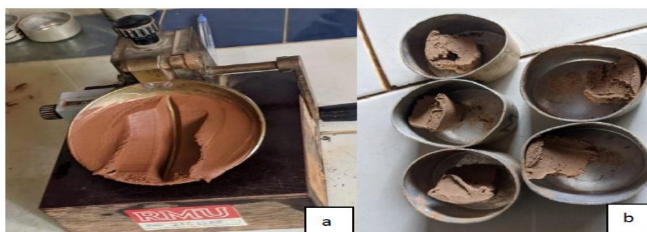
Fig 8 a) Casagrands apparatus (b) Samples removed for oven drying.
