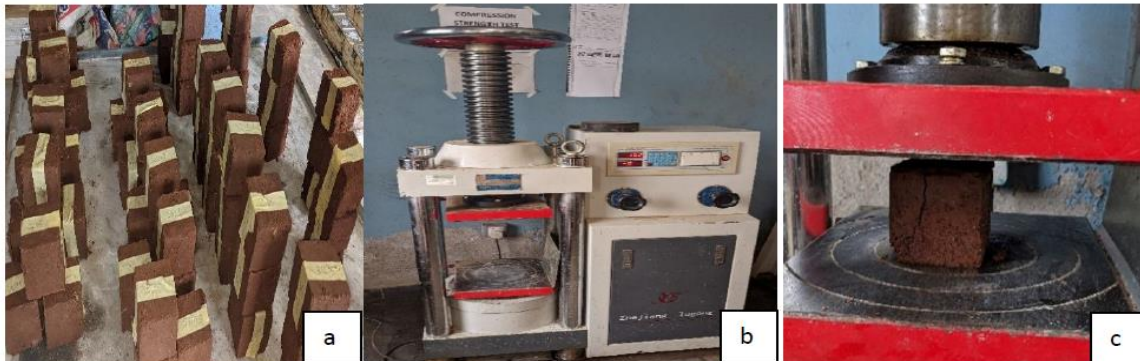
Figure 12 a) Samples ready for crushing b) Compressive strength machine c) Failed specimen.
