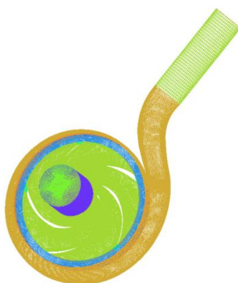
Fig. 1: Overall Model Mesh.
