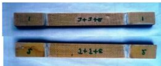
Fig 17 Tensile test Specimens Jute/Jute/Epoxy 3mm)
