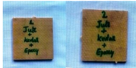
Fig 21 Compression test Specimens Jute/Kevlar/Epoxy (3mm)
