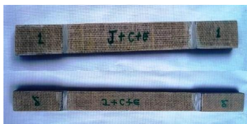
Fig 19 Tensile test Specimens Jute/carbon/Epoxy (3mm)
