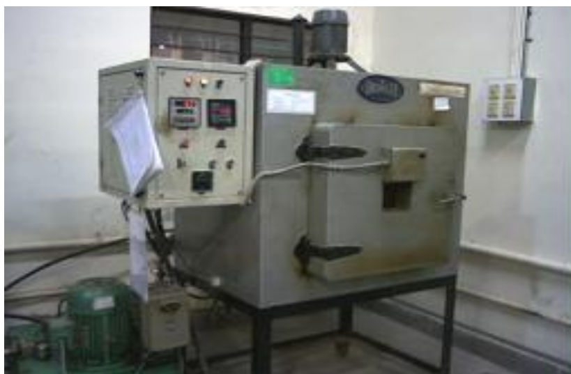
Fig 13 Post curing oven
