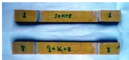
Fig 18 Tensile test Specimens Jute/Kevlar/Epoxy (3mm)
