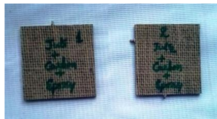
Fig 22 Compression test Specimens Jute/carbon/Epoxy (3mm)
