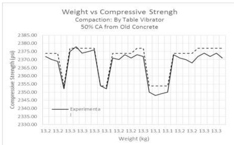
Figure 2: Graphical comparison of experimental and predicted compressive strength (TV)
