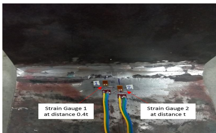
Figure 16: Specimen with strain gauges,
