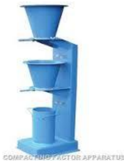
Fig 2: Compaction factor test.
