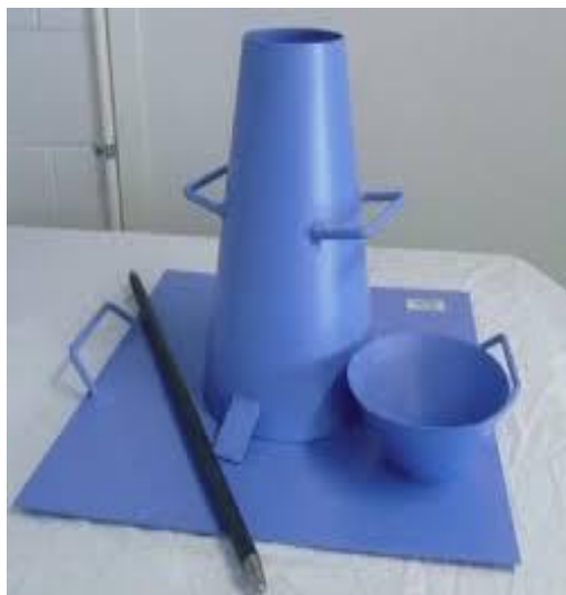
Fig 1: Slump cone test.
