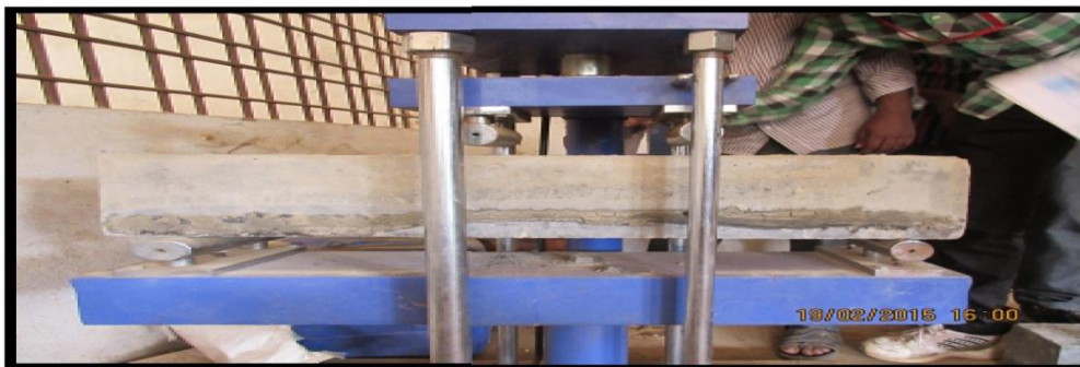
Fig 4: Flexural strength test.
