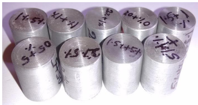
Fig. 11: Specimen for Corrosion test.
