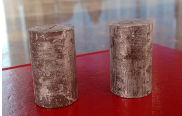
Fig. 13: Specimen after Corrosion.
