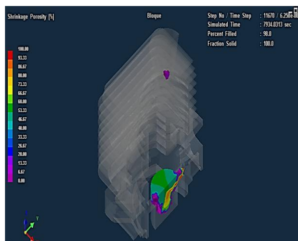
Figure 4: General porosity in the engine block.
