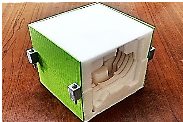
Figure 5: Silicone rubber molds to obtain wax patterns.
