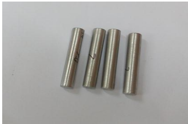
Figure 4.2: Wear Test Specimen.
