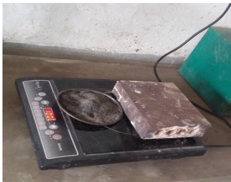
Figure f: The pre heat die.
