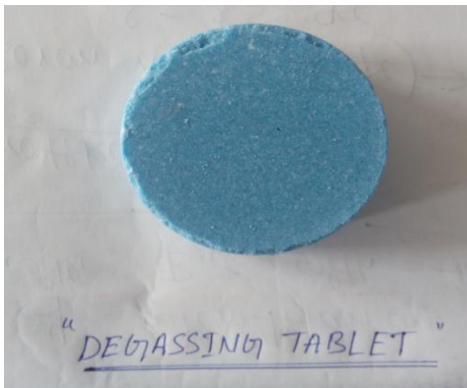
Figure g: The degassing tablet.
