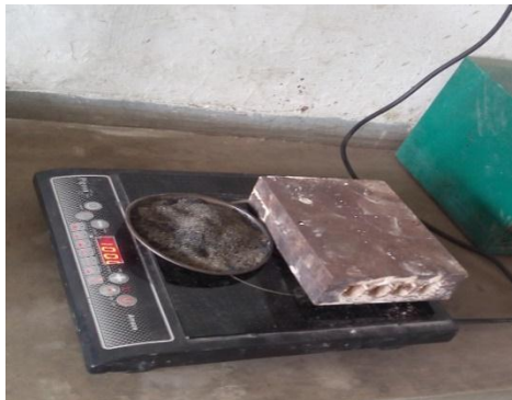
Figure f: The pre heat die.
