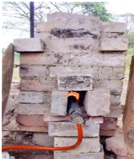
Fig 12: Furnace experimental set-up (Carbonization).
