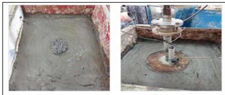
Fig. 6: Sample column after installation and plate load test.
