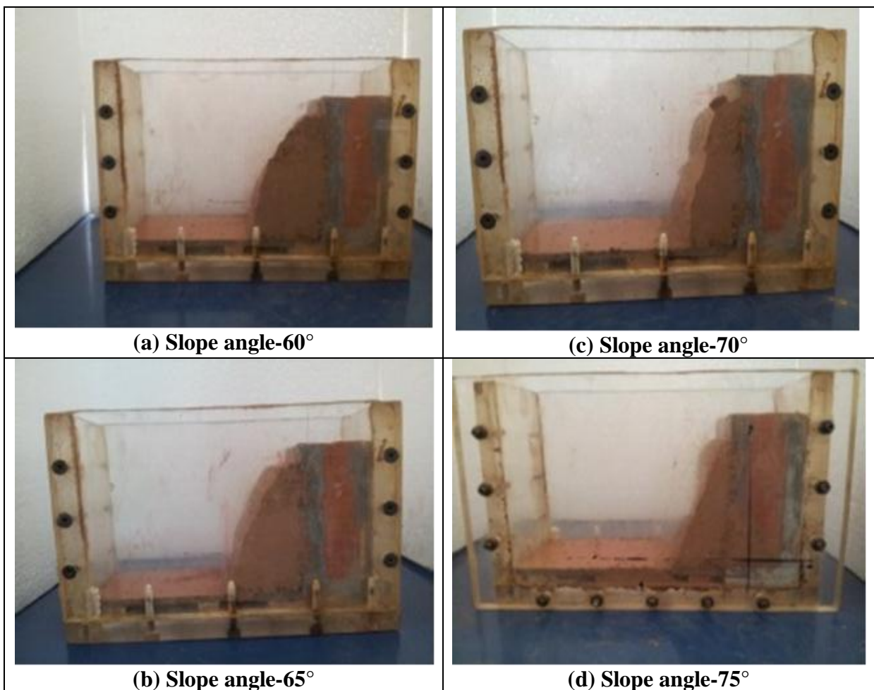
Figs. 10: a-d Slope condition for the Dry sample, without seepage and check of failure at every constant interval of angular velocity.
