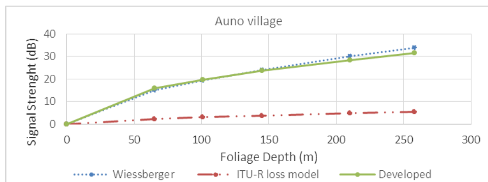
Figure 3: Signal Strength loss against foliage depth at Auno village of Wiessberger, ITU-R and developed (Maiduguri) model (Airtel) for wet season.
