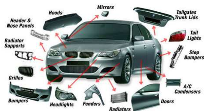
Figure 1: Application of plastics in automobile.
