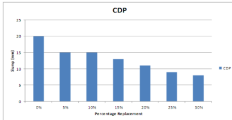
Figure 1: Bar chart for slump test of concrete produced using cow dung ash and cow dung powder.
