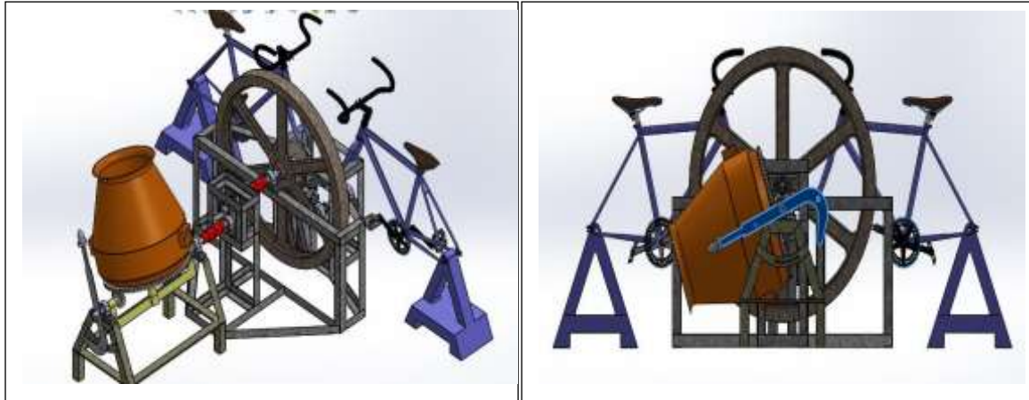
Figure 1: Schematic diagram of a HPFM energized process machine.
