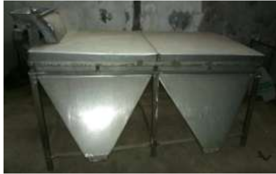
Figure 1: pictorial view of the vibrating screening machine.
