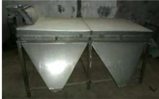
**Figure 1: pictorial view of the vibrating screening machine.**
