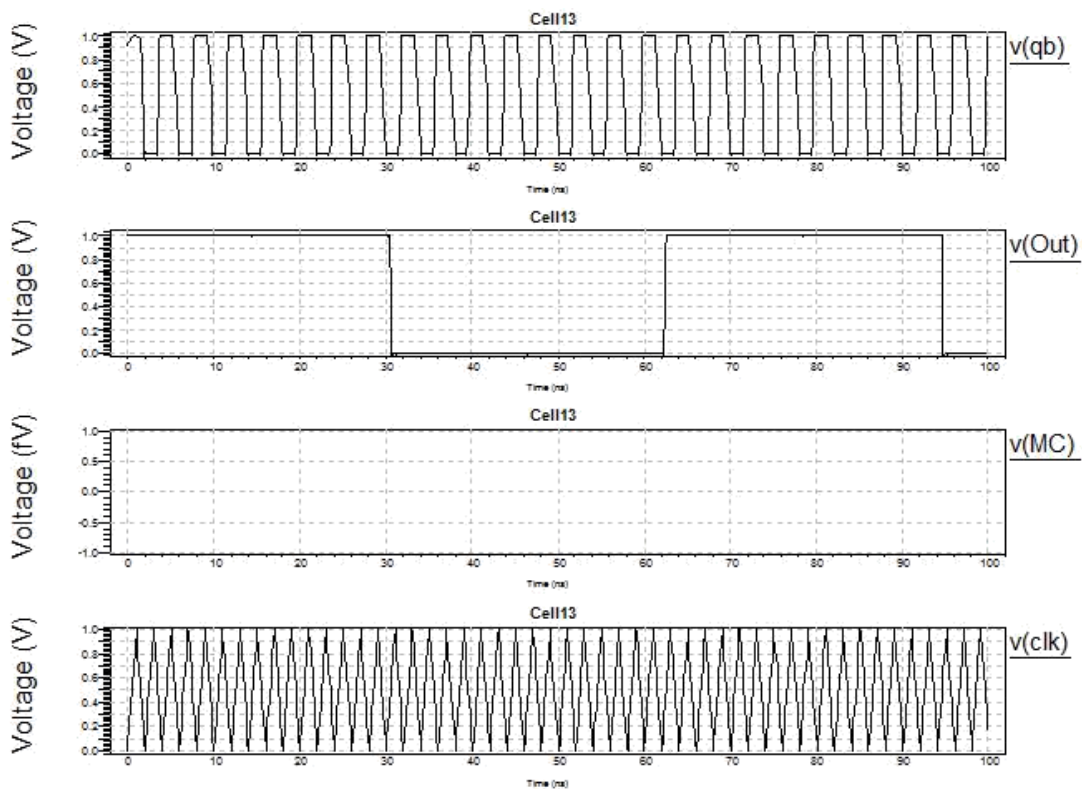
Fig. 9: Simulation waveform of divide by 33 counter.
