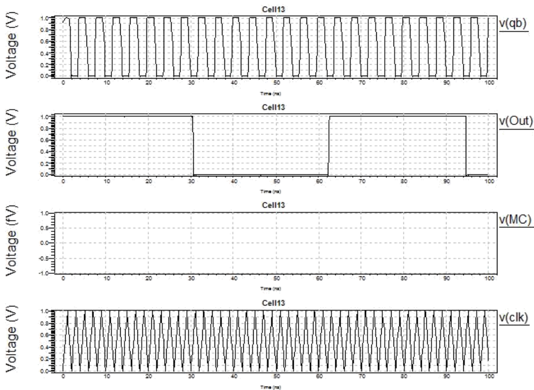
Fig. 9: Simulation waveform of divide by 33 counter.
