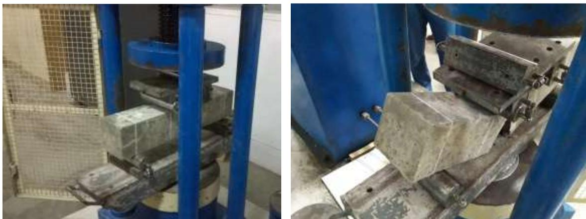
**Fig 8: Flexural strengths on Beam.**
