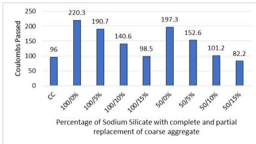
**Fig 13: Rapid chloride penetration test.**
