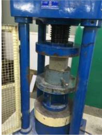
**Fig 2: Compression strength on cube.**
