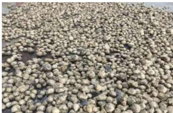
**Fig 1: Fly ash aggregate.**
