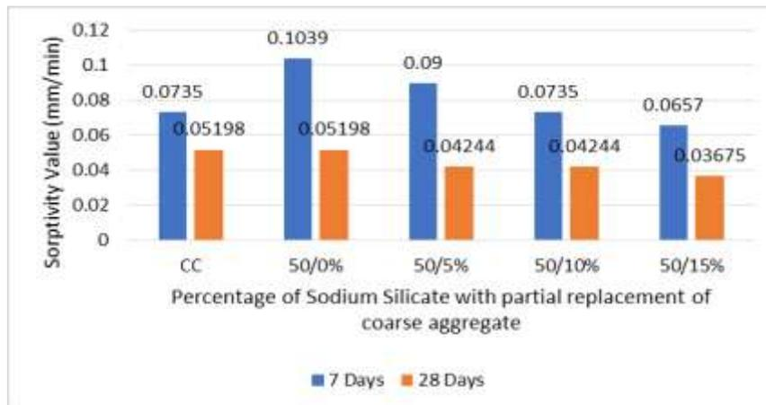
**Fig 14: Sorptivity test for partial replacement of coarse aggregate with various percentage addition of sodium silicate.**
