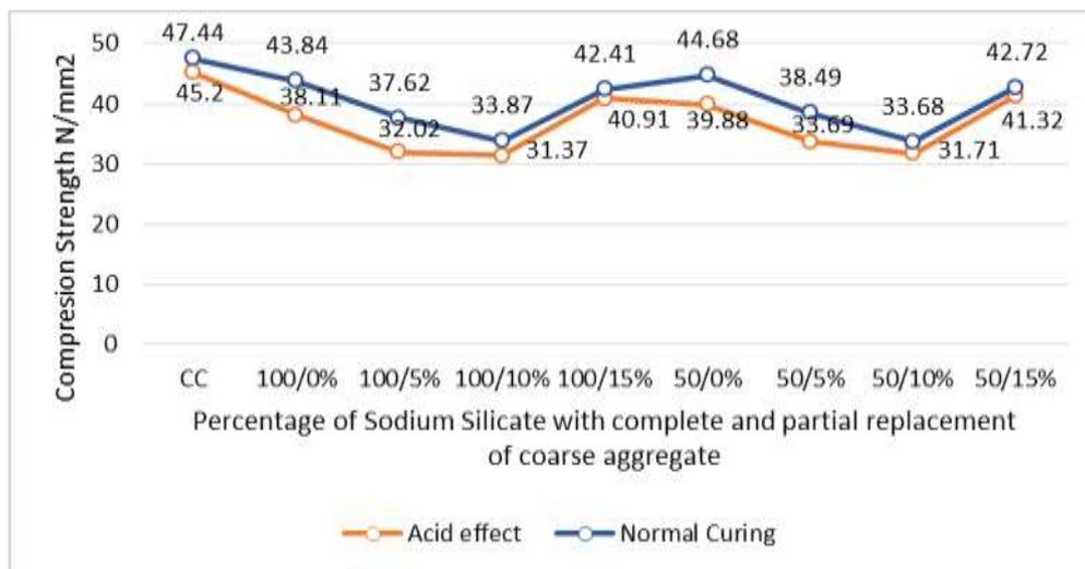
**Fig 11: Acid test.**
