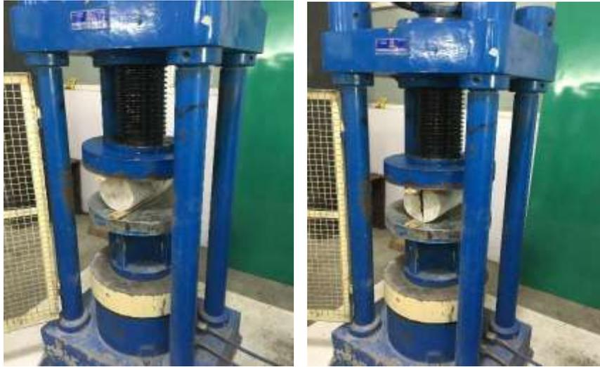
**Fig 5: Split tensile strength on cylinder.**
