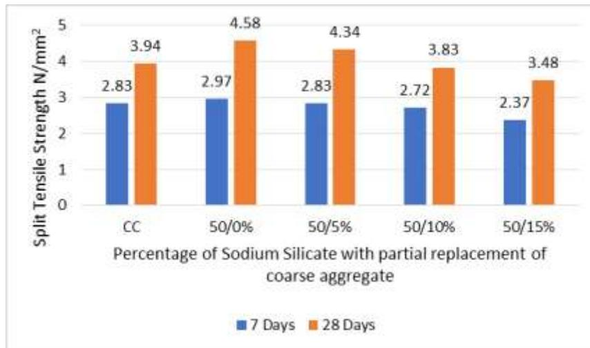
**Fig 6: Split tensile strength for partial replacement of coarse aggregate with various percentage addition of sodium silicate.**
