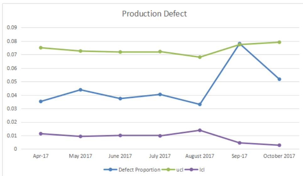
Based on the graph of the P control chart above, it was found that the production process at line Bending has gone well but in September 2017 it was above UCL which means it can be interpreted as an imperfect and uncontrolled production process. So there can be a deviation in the E-House Bending Production Line.
