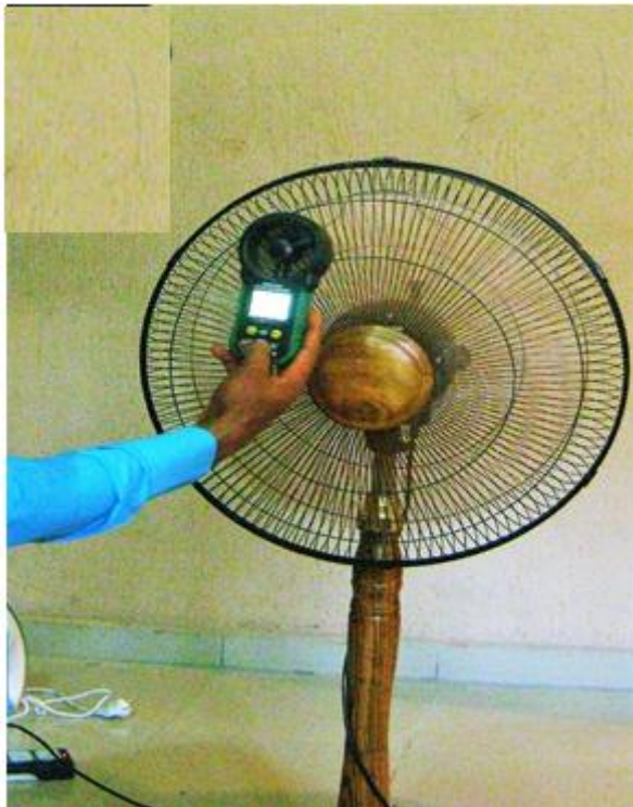
Figure 7: Positioning the Anemometer.
