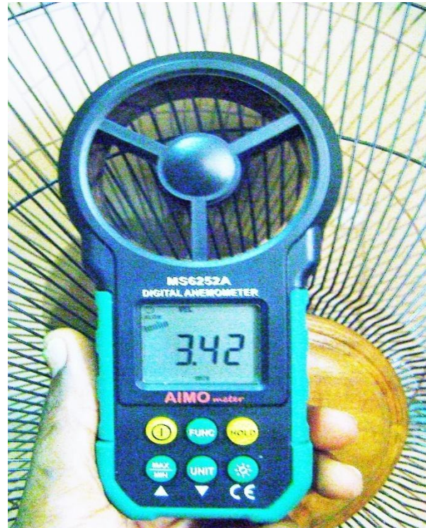
Figure 8: Taking reading with Anemometer.
