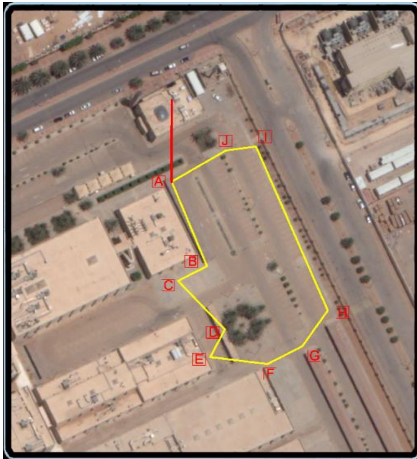
Fig. 4: Traverse Control and Test Points.
