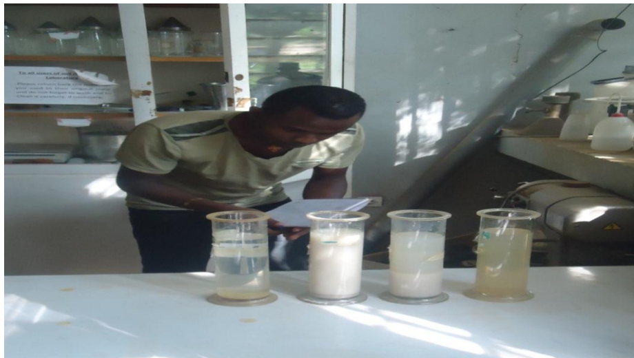
Fig. 3: View of conducting double Hydrometer Test on dispersive soil.
