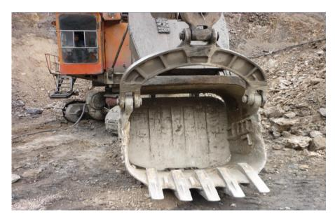
Fig. 3: General view of the front wall of the bucket with established teeth on it. CONCLUSIONS
