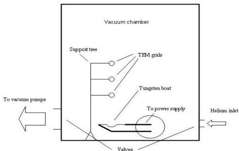
**Figure 7: Inert gas condensation system.**
