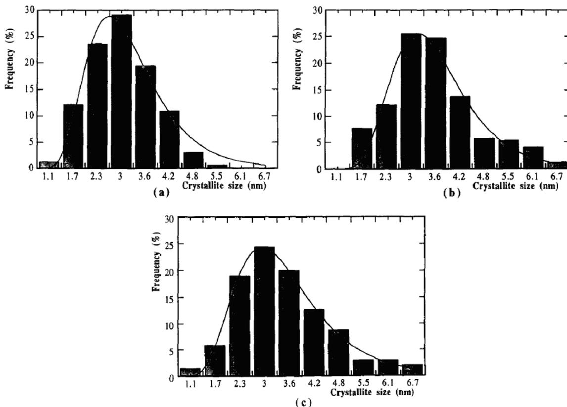
**Figure 3: Particle size distribution of ceria particles, a) particles on the substrate, b) particles on the walls near the substrate, c) particles in the surrounding of the evaporating boat.**
