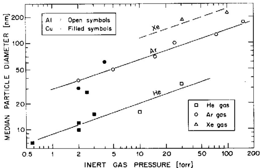
**Figure 2: Al and Cu particle sizes made in various inert gases.**
