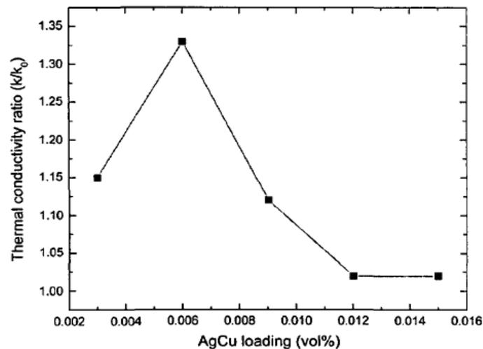
**Figure 12: Thermal conductivity vs. Ag-Cu nanoparticles volume in a fluid.**
