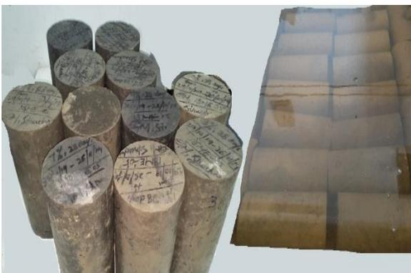
**Figure 3: Curing of Specimens.**
