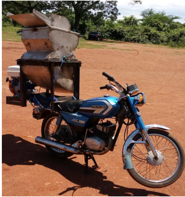
Figure 5: Modified NCAM Cassava Grater on Motorbike.
