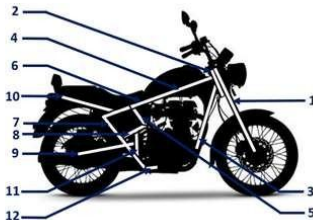
Figure 1: Schematic diagram showing elements in a Royal Enfield Thunderbird 350 chassis.
