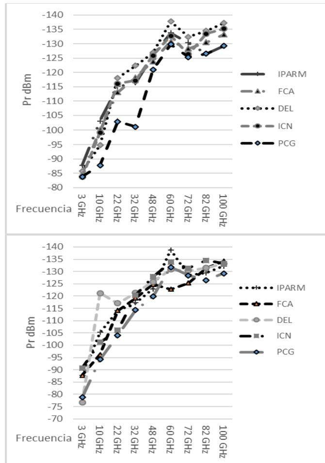
**Figure 4: Loss of signal in free space (up operator X-down operator Y).**
