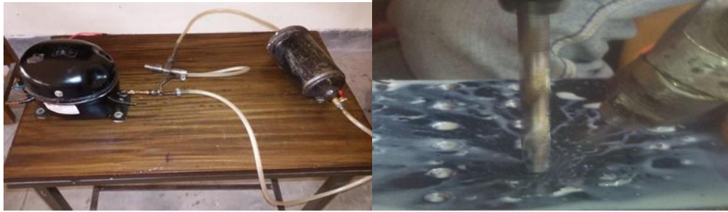
Figure 2: The minimum quantity lubrication system set-up and its application.
