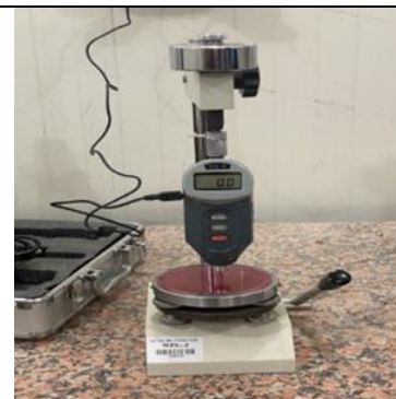
Fig. 9 (shore D) test device
