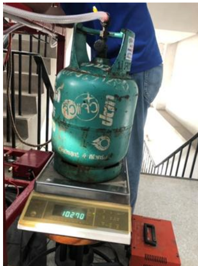
Figure 4: LPG fuel consumption measurement.
