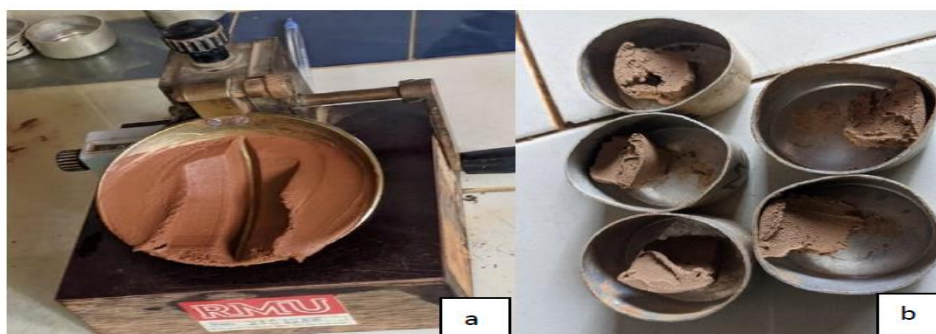
Fig 8 a) Casagrande's apparatus (b) Samples removed for oven drying.
