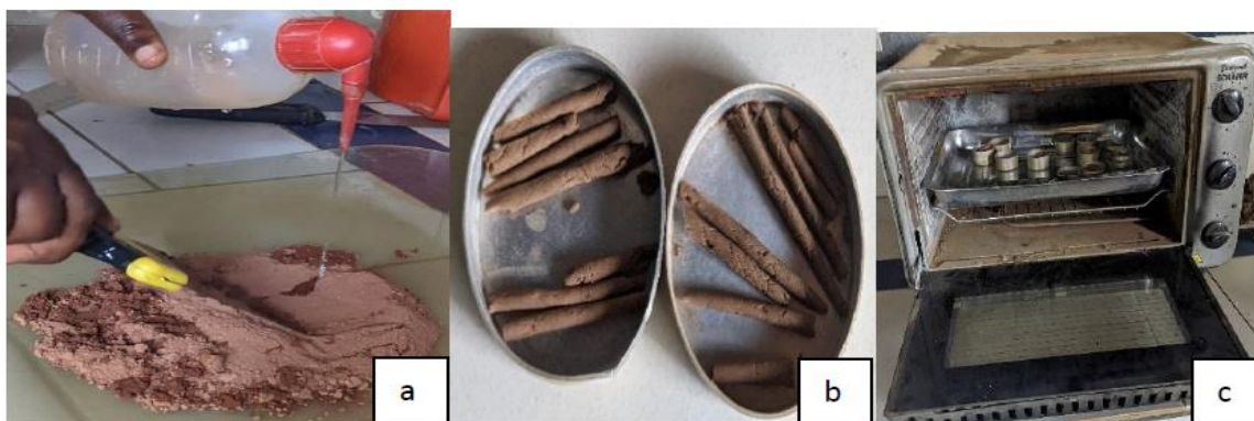
Figure 9: a) Soil preparation for plastic limit test b) Samples to be put in the oven c) Oven drying.
