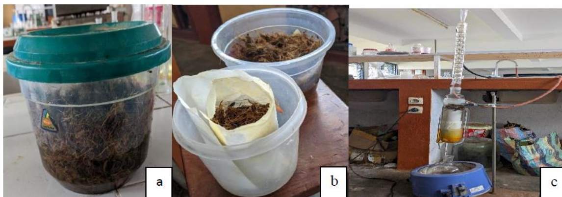
Figure 4 a) Maceration process of OPMF b) Filtering of and Preparation for soxhlet process c) Soxhlet extractor.
