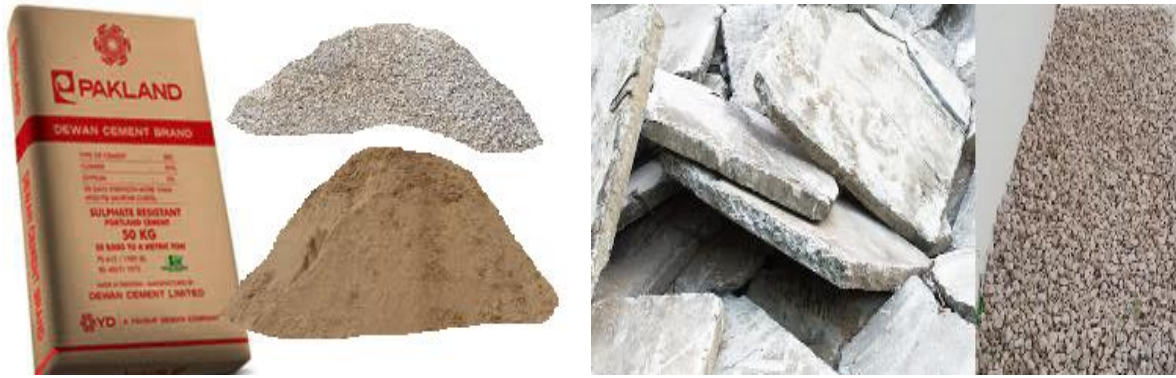
Figure 1: Concrete ingredients. Figure 2: Demolished Waste and Recycled aggregates.
