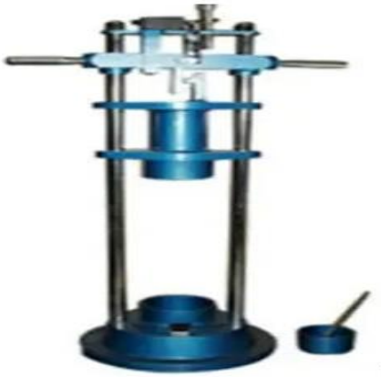
Figure 3: Impact value test.
