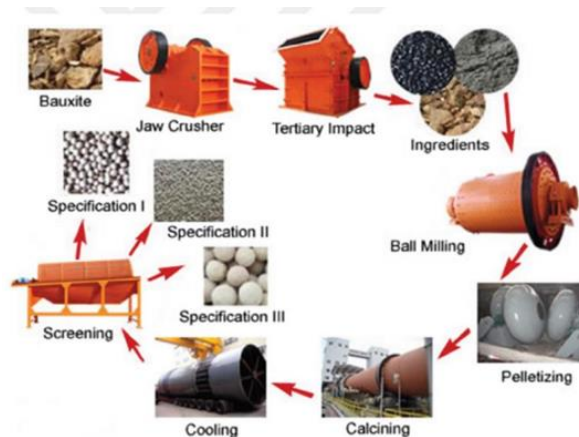
Figure 1: LECA production flow chart.
