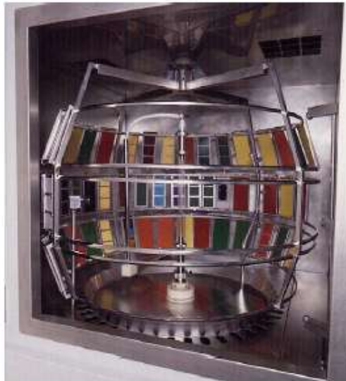
Figure 4: Layout of the samples in side the weather-Ometer.
