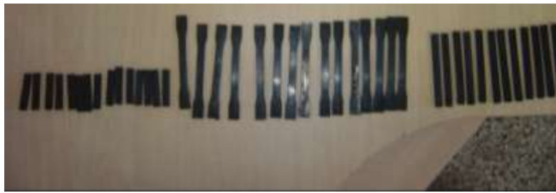
Figure 6: Test samples as per ASTM standard.
