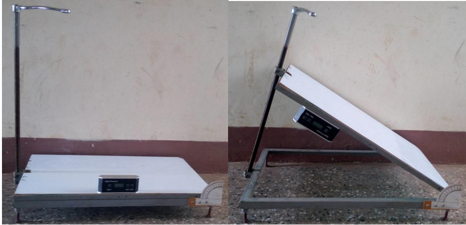
Figure 4: Manufactured Inclino-Tribometer used.
